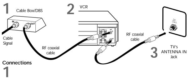
Connect a Cable signal to the IN Jack on the Cable Box/DBS.
